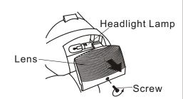
4 Remove the lamp by pushing it gently in the direction of the arrow and then turning it counterclockwise.
